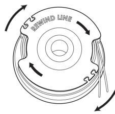
Lock the cutting line in the slot when not use.
